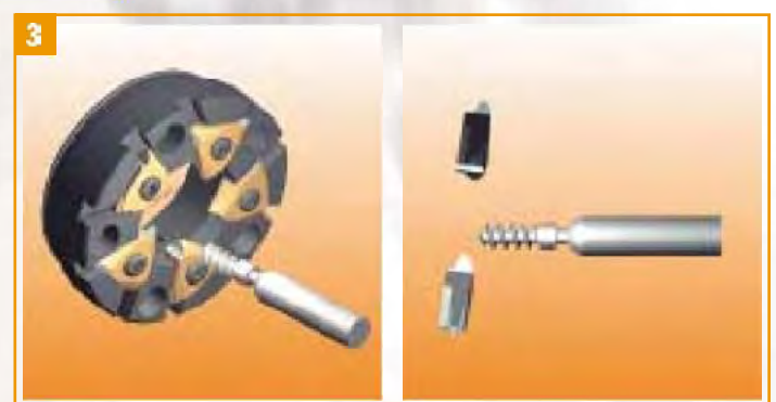
The required thread length is achieved. The whirling spindle moves first back radially and then axially thereafter.
