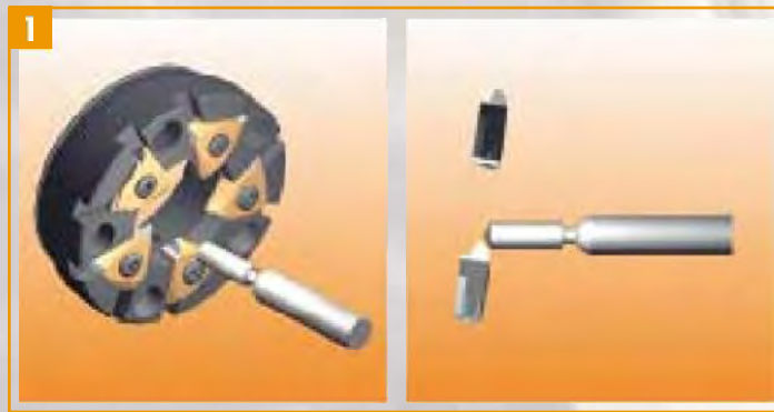
The thread whirling spindle is set up in front of the work piece and rotates at high speed. The work spindle rotates at a lower speed in the same direction.
