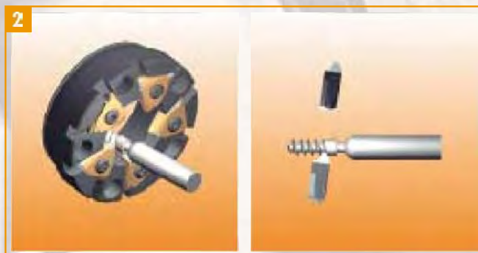
Thread whirling begins. The thread is achieved through a rotating motion of the C-axis and a longitudinal motion of the Z-axis, only one of the whirling spindle's cutting edges is in operation during this process.
